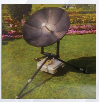
The reflector manufactured using Carbon fiber reinforced Plastic (CFRP) in segments and joined together to form a Parabolic Reflector.
